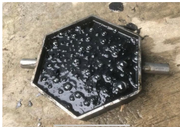
Gambar 4.4 Pencetakan Paving Block
