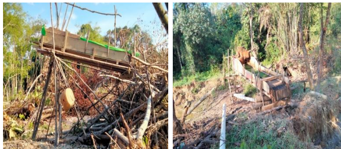
Gambar 4. Kiyang/Biduk ( Sluice Box )
